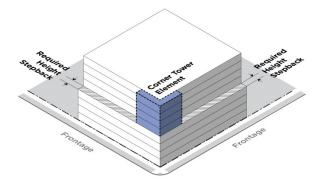
**Stepback**. A stepback is the required additional distance that upper stories of a structure must be recessed from the facade of the stories below. A required stepback must continue through all upper stories once established, though it may be increased from any required minimums on any stories.
