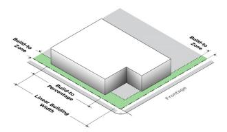
**Build-To Zone (BTZ).** A build-to zone (BTZ) is the area on a lot, measured perpendicularly from the lot line, within which a structure must locate. A build-to zone sets a minimum and maximum dimension within which the building facade line must be located (e.g. 0-5'). Facade articulation, such as window or wall recesses and projections are not counted as the building facade line, which begins at the applicable facade wall.
