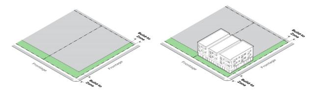
**Building Line.** The vertical plane along a lot where the building's facade is located. Upper story building lines relate to that part of the facade that requires a stepback.
