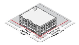
**Building Length.** Building length is measured as the length of the facade abutting a frontage type. Passageways, breezeways, ground floor passages, and similar building connections are included in the calculation of total building length.
